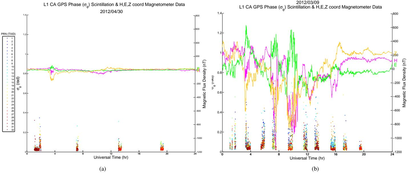
Fig. 6. Geomagnetic activity on fluxgate magnetometer and low rate GPS phase scintillation on CASES recorded at the AAL-PIP South Pole Station 4 during (a) a 'quiet' day and (b) a storm day.
