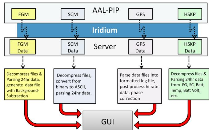
Fig. 2. Block Diagram of the overview of the work cycle, the file transfer, data handling, and display in the Graphical User Interface.
