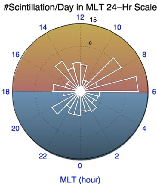
Fig. 8. Cumulative number of scintillations per hour during high rate collection for the test period
